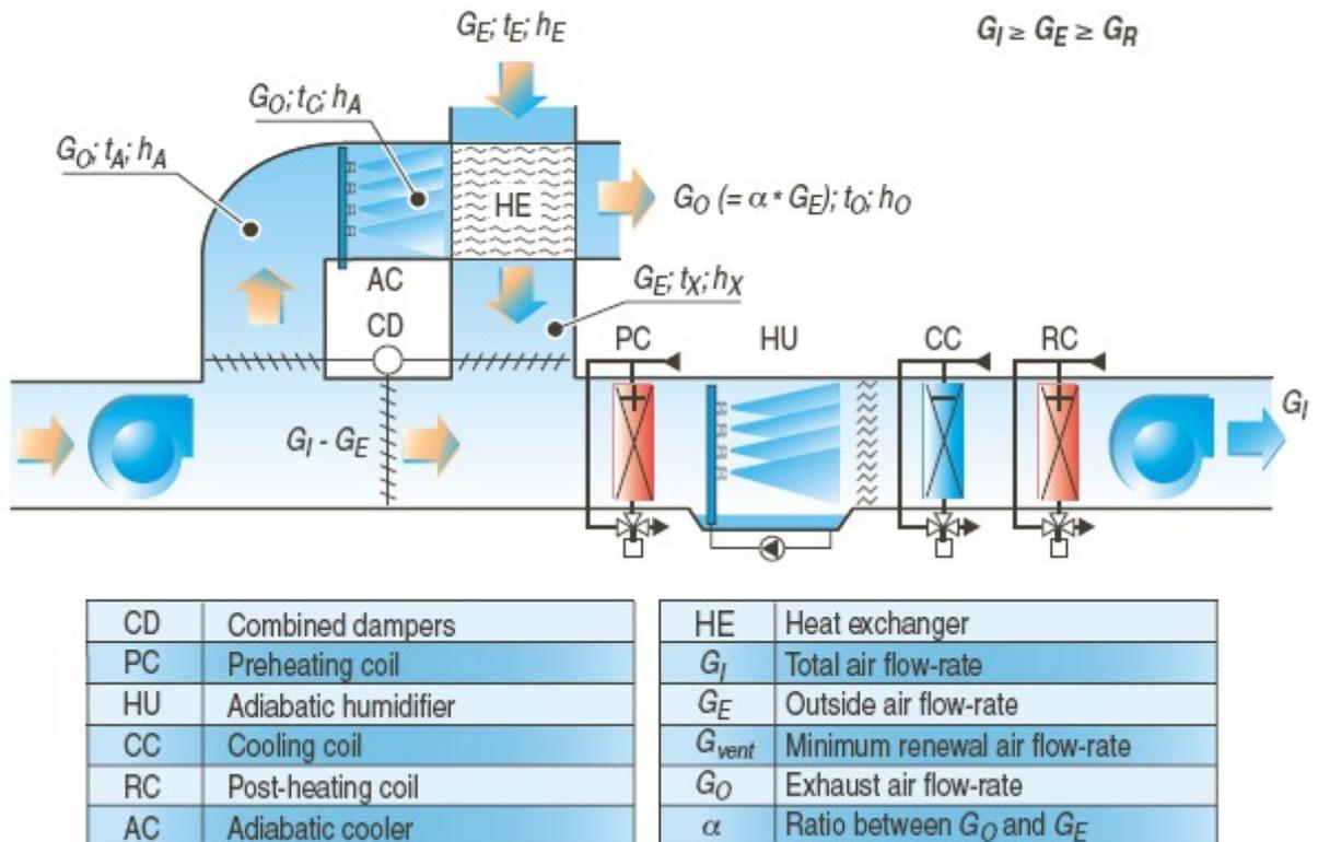
Fig. 3 Possible diagram of an installation for indirect evaporative cooling
