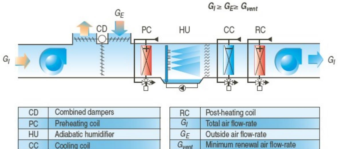
**Fig. 2** -System diagram for direct evaporative cooling with motor-driven dampers to adjust the recirculation of air in favour of renewal air
