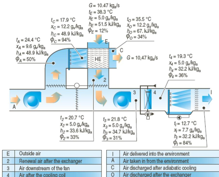
Fig. 4 Diagram of an indirect and direct evaporative cooling installation developed in California
