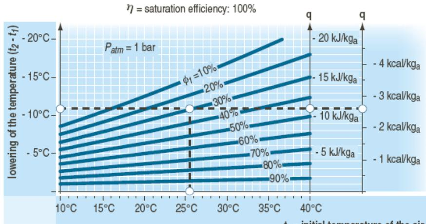
**Fig. 1** - Specific cooling energy ( $q$ ) and lowering of the temperature (final temperature  $t_2$  – initial temperature  $t_1$ ) obtainable by adiabatically humidifying air, with a saturation efficiency  $\eta = 100\%$ , according to the initial temperature ( $t_1$ ) and the relative humidity ( $\phi$ )
