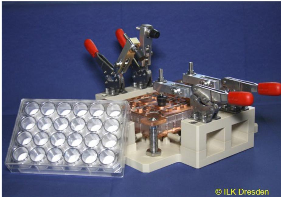
**Fig.1:** Multiwell RACK for cryopreservation of allogeneic transplants
