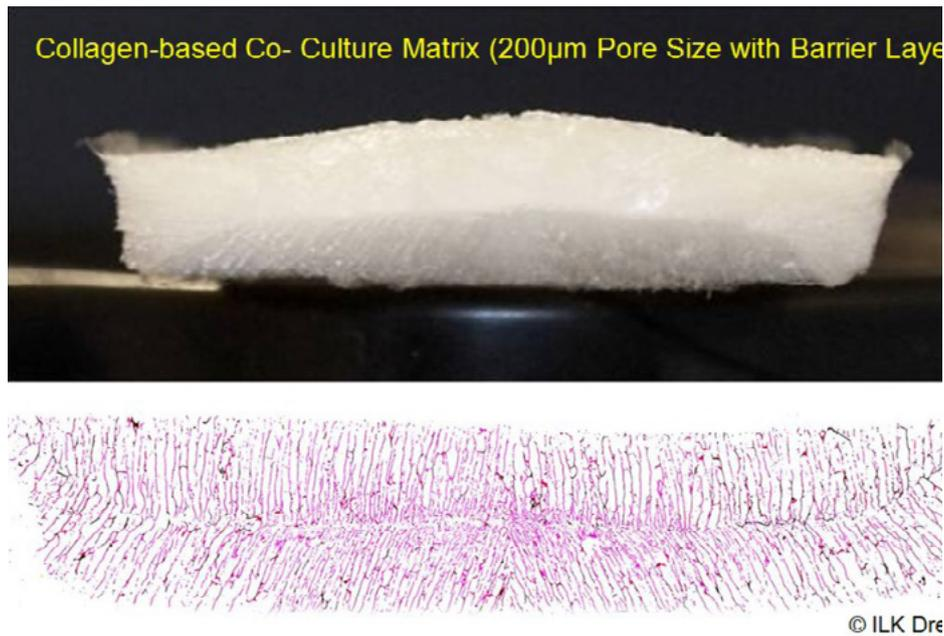
**Fig.2:** Biodegradable carrier material compound with bi-layer-structure from collagen manufactured by MBIT-Freeze-drying process
