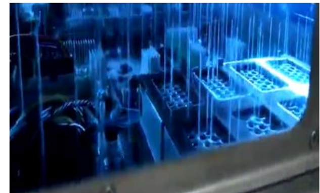
Spray liquid cooling
